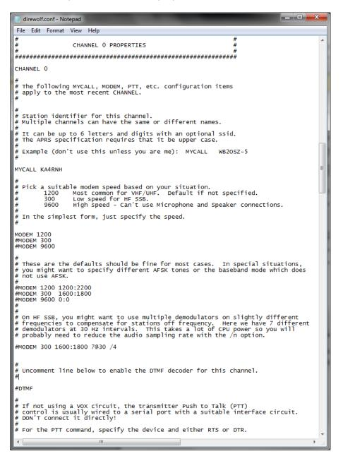
Since I am only using one channel. I set the call sign to my own call sign. Then I uncommented out the "MODEM 1200" line. As you can see by the other examples you modify the behavior of the modem parameters in a variety of ways. There is no need for a DTMF decoder. Not show are the PTT parameters, because I was using VOX, however those can be set for each channel too.
