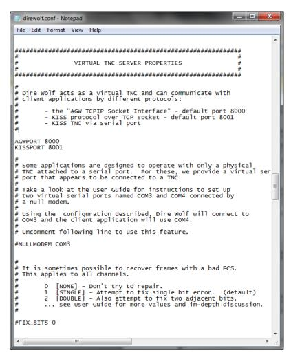
As you can see this is where the AGWPORT is set and the KISS network port are set. I left them to default. Note the AGWPE port number is the same port number as specified in the Outpost Interface->AGWPE tab. Notice also that this is where I uncommented the "NULLMODEM COM3" and set the value for the virtual null modem when I was trying to get Outpost to work via a COM port. I commented this line out when I switched to using the AGWPE network port.
